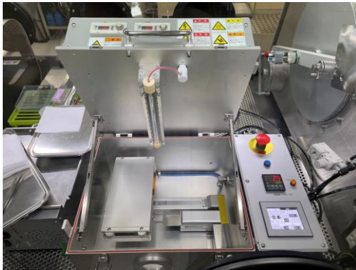
VUV irradiation system in glovebox
