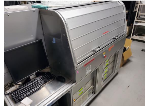
Continuous driving test for OLEDs
