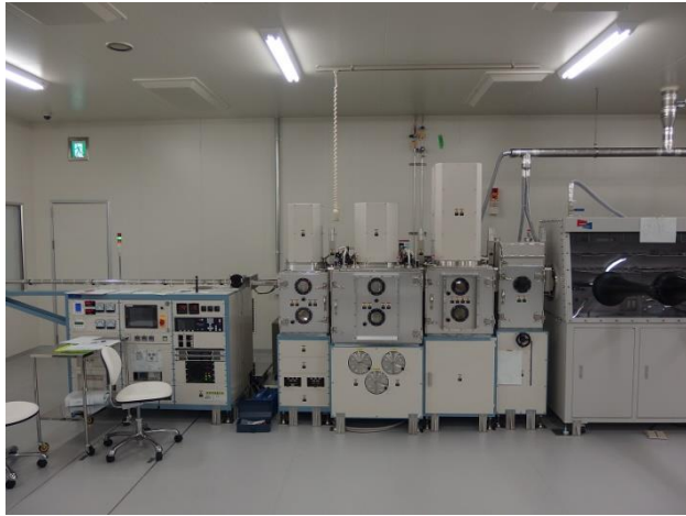
Vacuum vapor depo., Sputter Substrate ~200x200 mm
